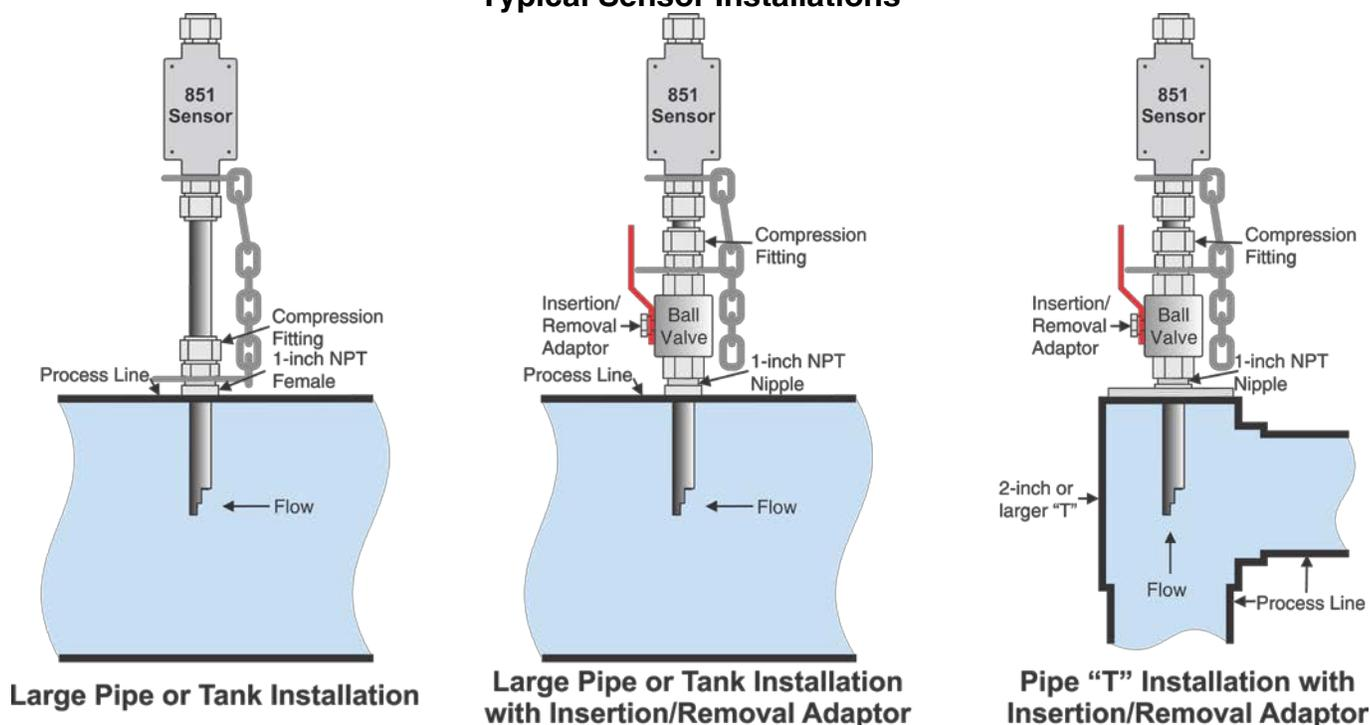
**Transparent Lines:** If the sensor is to be used in a transparent (e.g., glass, PVC, acrylic, etc.) process or sample line, the pipe must be wrapped with tape to prevent ambient light from entering the pipe and affecting the readings. Wrap the pipe for a distance of at least five pipe diameters from the sensor. **Black PVC electrical tape will not block light sufficiently.** Use an aluminum tape or wrap any tape over a metallic foil.
